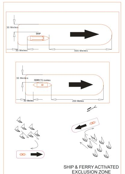
Be mindful of larger ships' bow flare. When closing any vessel, to prevent being overrun ensure you remain within sight of the Master / Officer of the Watch on the vessel's bridge. Beware of overhanging bows and other parts of ship that might obstruct this line of sight. This means that your vessel may disappear from sight inside 500m from the bows of very large ships.
